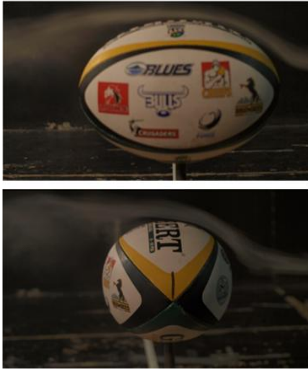
Fig 8. Flow structure (smoke) around ball 0° and 90°
