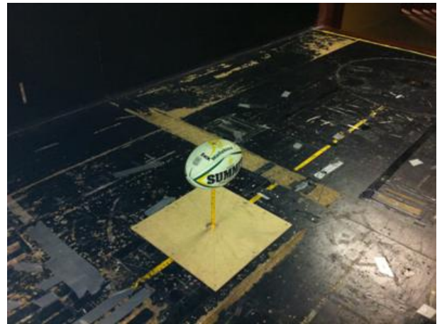
Fig 2. Orthogonal view of experimental set-up with rugby ball in wind tunnel's test section
