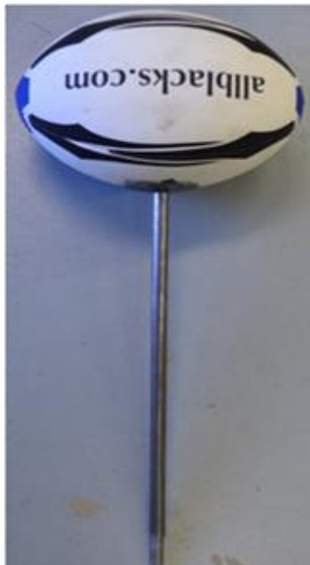
Fig 6. Specially designed mounting sting
